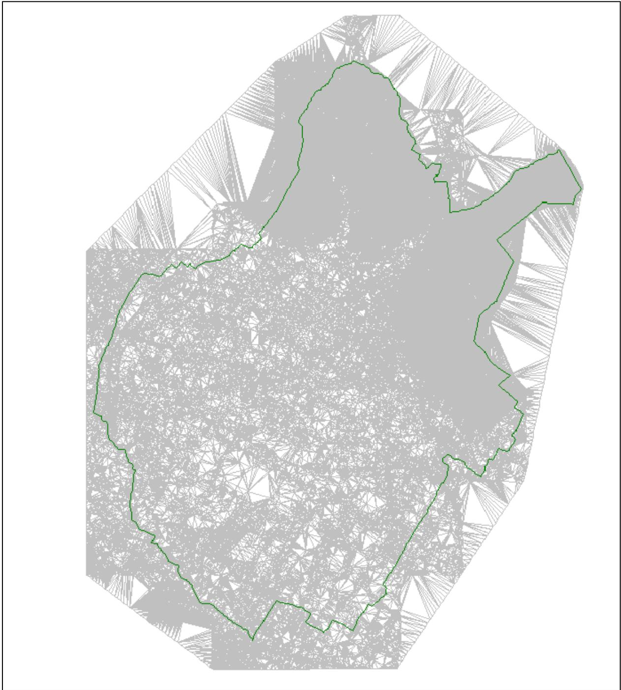
**Figura 14 - Triangoli del Digital Ground Model (DGM) in vista planimetrica**
